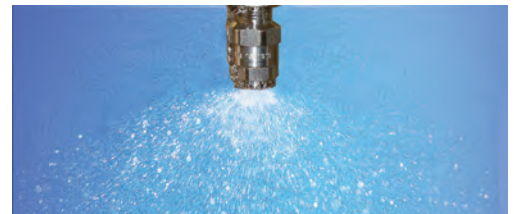
Outdoor moisture attack is simulated by spraying pure water onto specimens.
